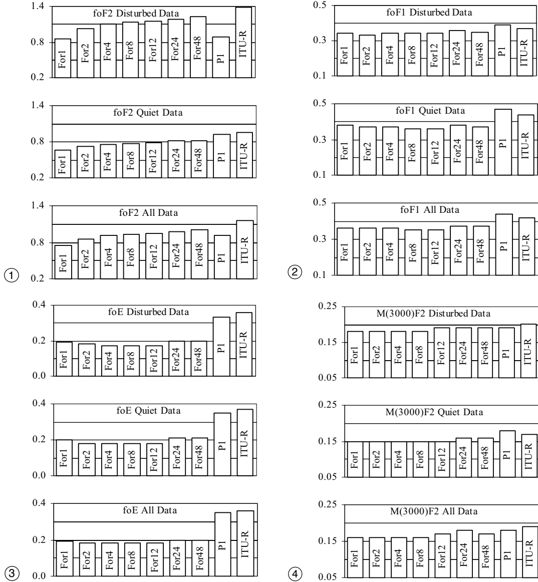
Fig. 1. Bar chart created for RMS errors for f_oF_2 characteristic, for disturbed data (upper panel), quiet data (middle panel), and for all data together (lower panel). Autocovariance forecasting method: For1, 1 h ahead For2, 2 h ahead, etc. Persistence: P1.
