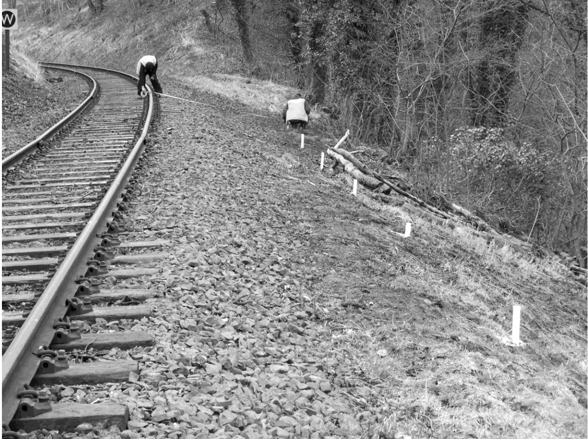
Figure 5: Setting out tell-tales in a priority area
