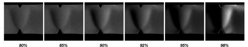
The degree of knife edge cutoff is taken as the ratio of unobscured width to total width of the source image and its effect for several cutoff levels can be seen above. Increasing the cutoff leads to increasing contrast changes. The dark regions above 95% cutoff results from strongest refractions that cause the displaced image to move entirely onto the knife edge. As a result, a change in image illuminance is no longer produced; this effect is known as *underanging* [1].
