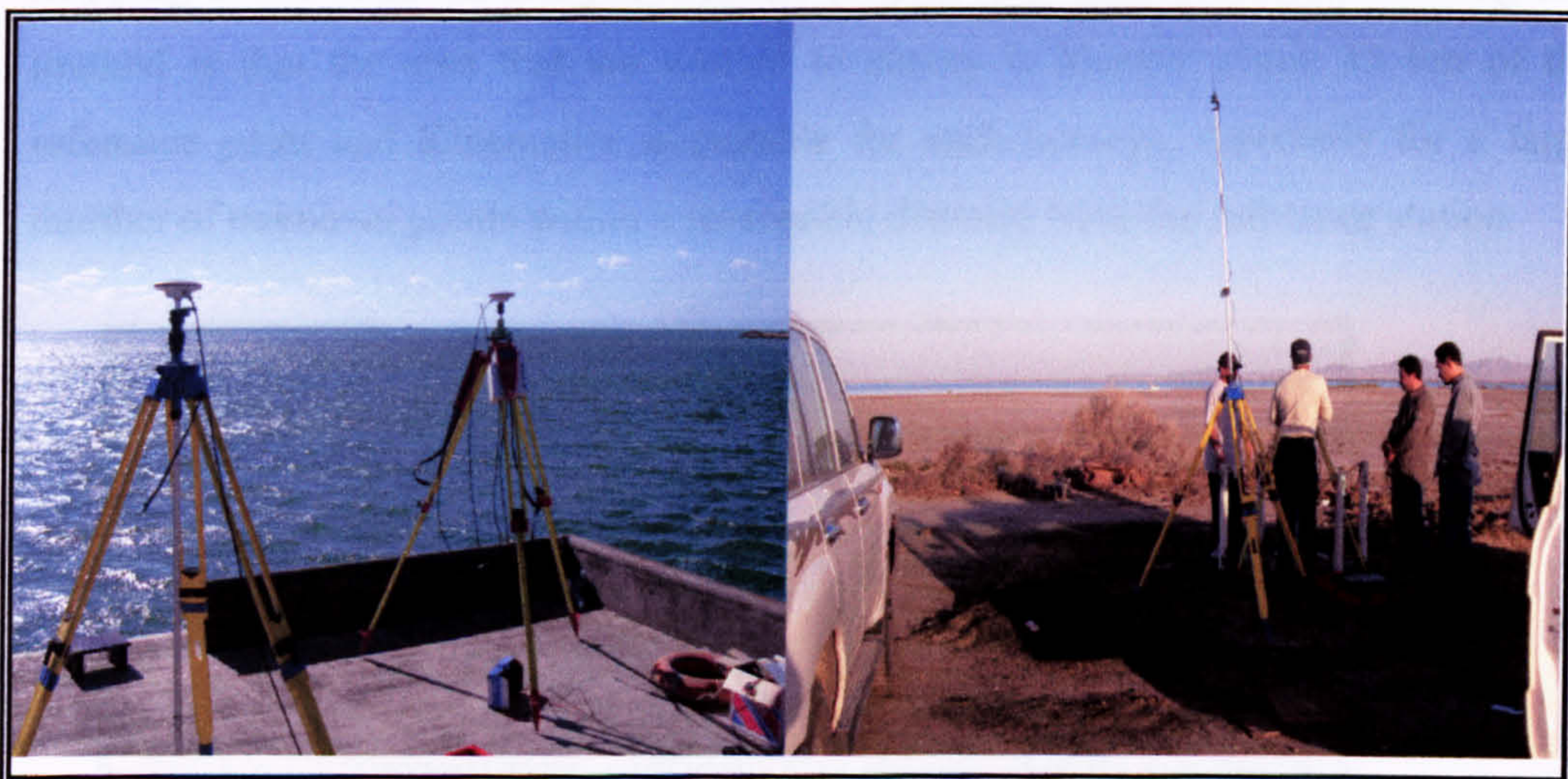
Figure 4.6. Field photographs showing the GPS static processing method
