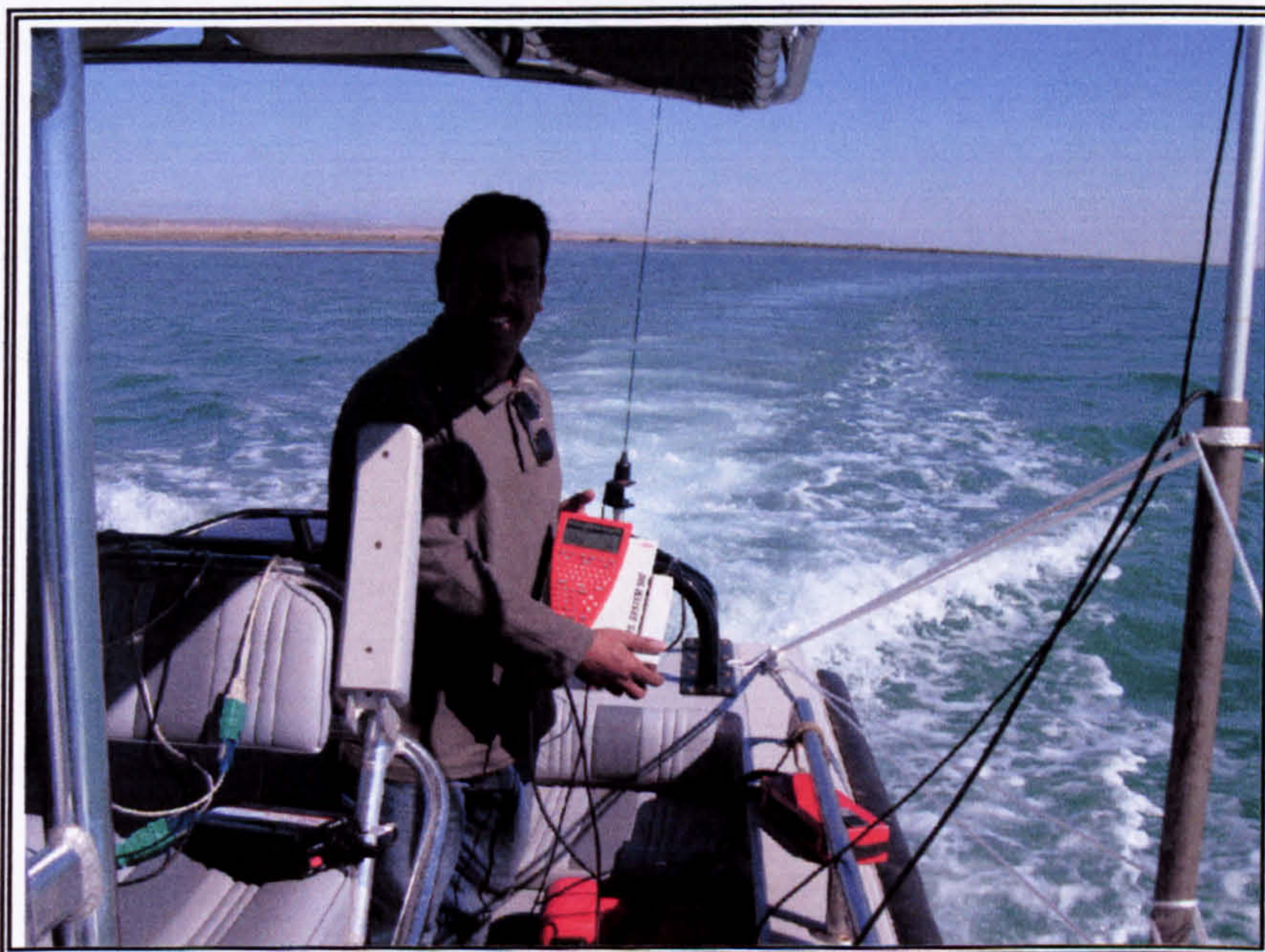
Figure 4.8 The RTK GPS equipment used during the hydrographic survey.
