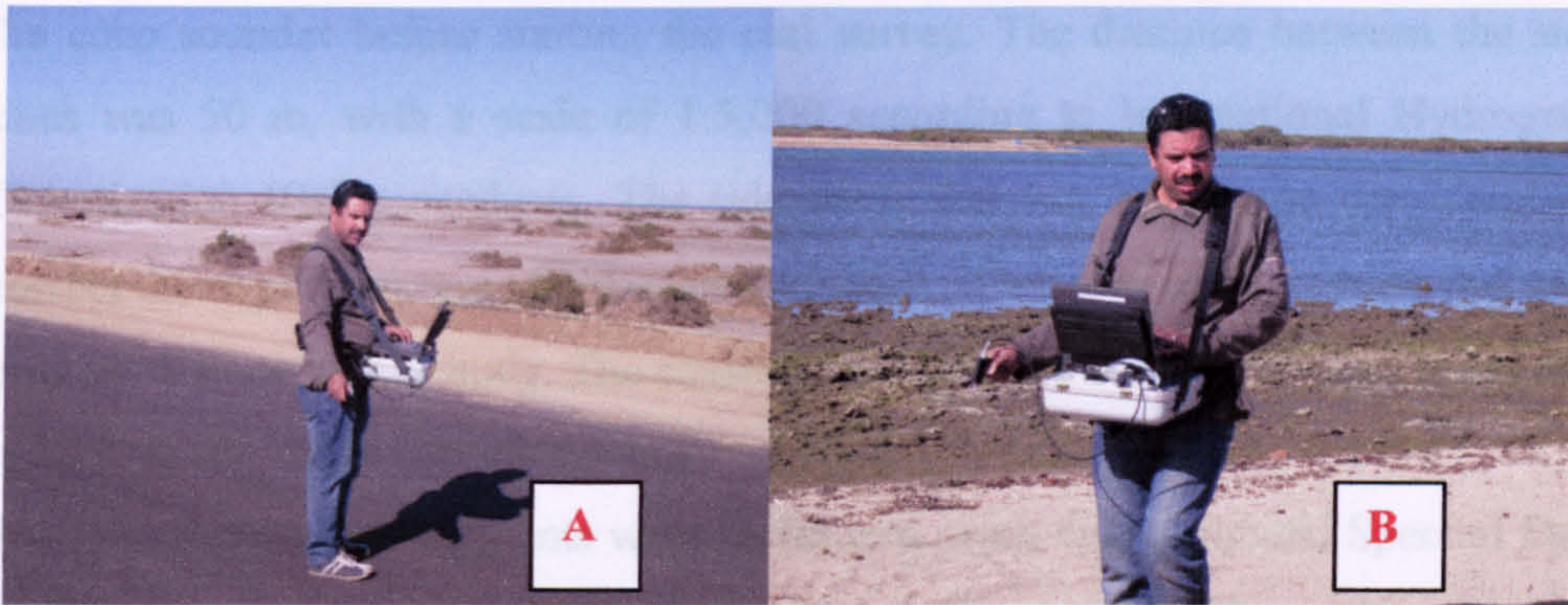
Figure 4.16. Practical spectral measurement. (A) Dark object (Asphalt). (B) Bright object (Sand).
