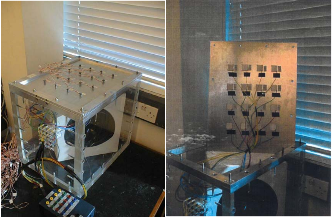
Figure 5: A smart panel with sixteen decentralised velocity feedback units, using rectangular piezoelectric patches and matched velocity sensors. (From Ref. 56)
