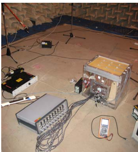
Figure 51: The experimental test setup for the measurements of the radiated sound power in the anechoic chamber.
