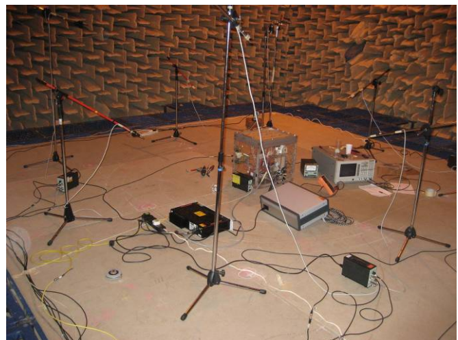
Figure 51: The experimental test setup for the measurements of the radiated sound power in the anechoic chamber.
