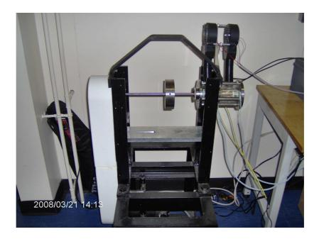
Figure 7- 3: The Antagonistic SMA/Composite Smart Bearing Test Rig
