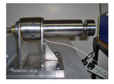
Figure 7-7 : Close-up of the Piezoelectric Exciter
