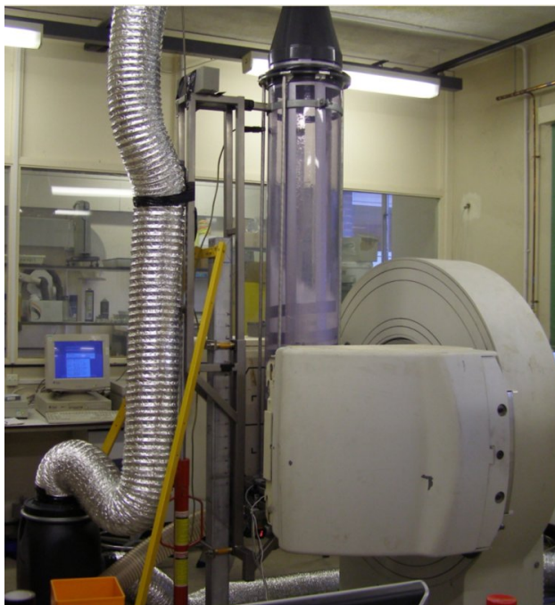
Figure 6.1: ADAC camera used to study a fluidised bed
