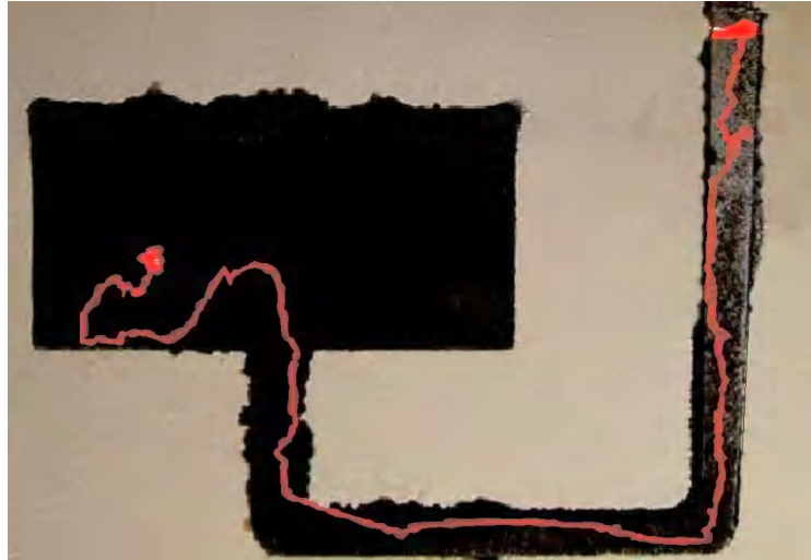
Figure 7.15: Trajectory of a particle introduced into liquid metal during casting
