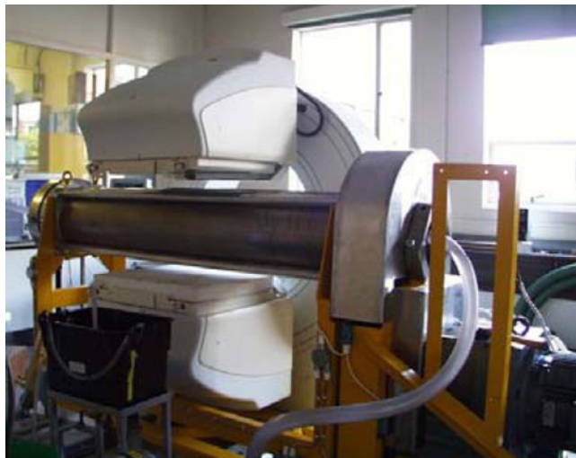
Figure 6.2: ADAC camera used to study a scraped surface heat exchanger
