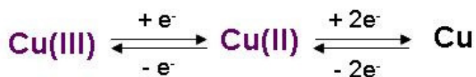
Figure 93. Scheme of the electrochemical behaviour of the copper complex on GC, in alkaline media. The purple colour denotes complexed species.
