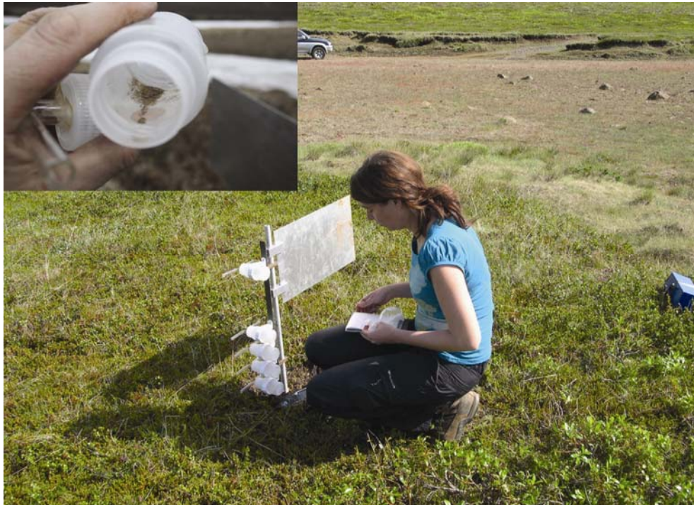
Figure 23- Sediment trap and insert a sample bottle showing the sediments collected by the sediment trap at Baldursheimur after a year.
