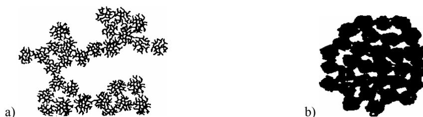
**Figure 1.7.** Scheme of base-catalyzed gel (a), desiccated xerogel (b).
