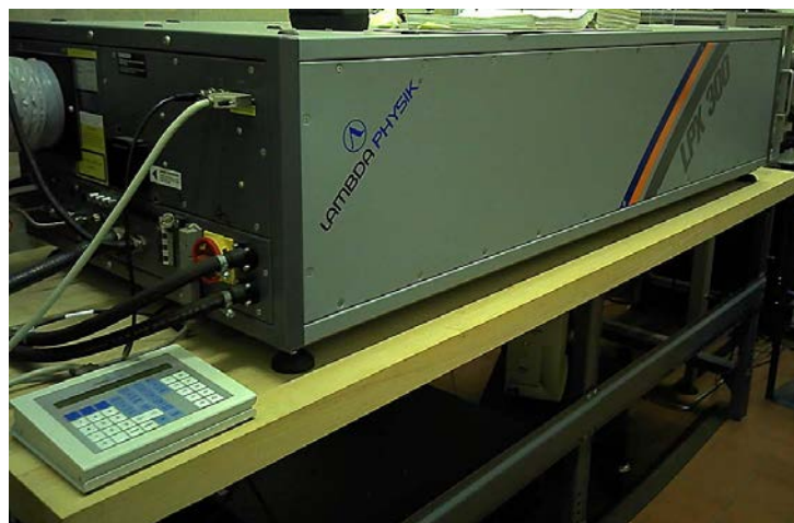
Figure 3-4 Lambda Physik LPX 300 laser system used in this project
