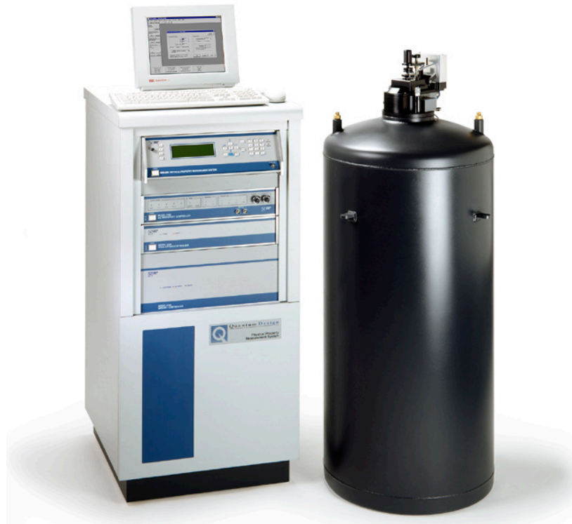
Figure 3-12 MPMS system used in this project, with DC magnetic field up to 6 T
