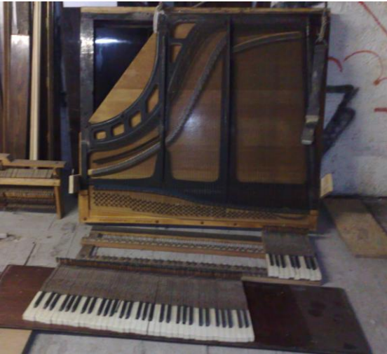
Figure 4. The piano in bits, showing how I planned to re-attach the keyboard
