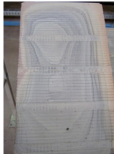
Fig. 35: Color effects on brick surface due to the use of foundry sands
