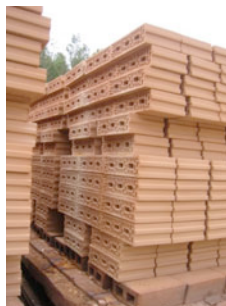
Fig. 43: Open setting on kiln car at Ziegel Gasser Mattoni GmbH S.r.l.
