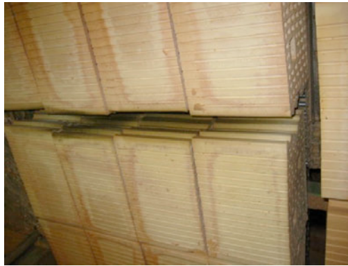
Fig. 70: Ziegel Gasser Mattoni GmbH S.r.l. brick with de-coloration on visible surface
