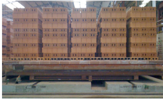
Fig. 13: Bricks on a kiln car in a modern plant (VELA S.p.A. Fornaciai Bologna)
