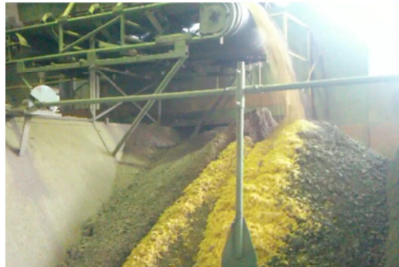
Fig. 47: Glass fiber is added to the mix (VELA S.p.A. Borgonato)
