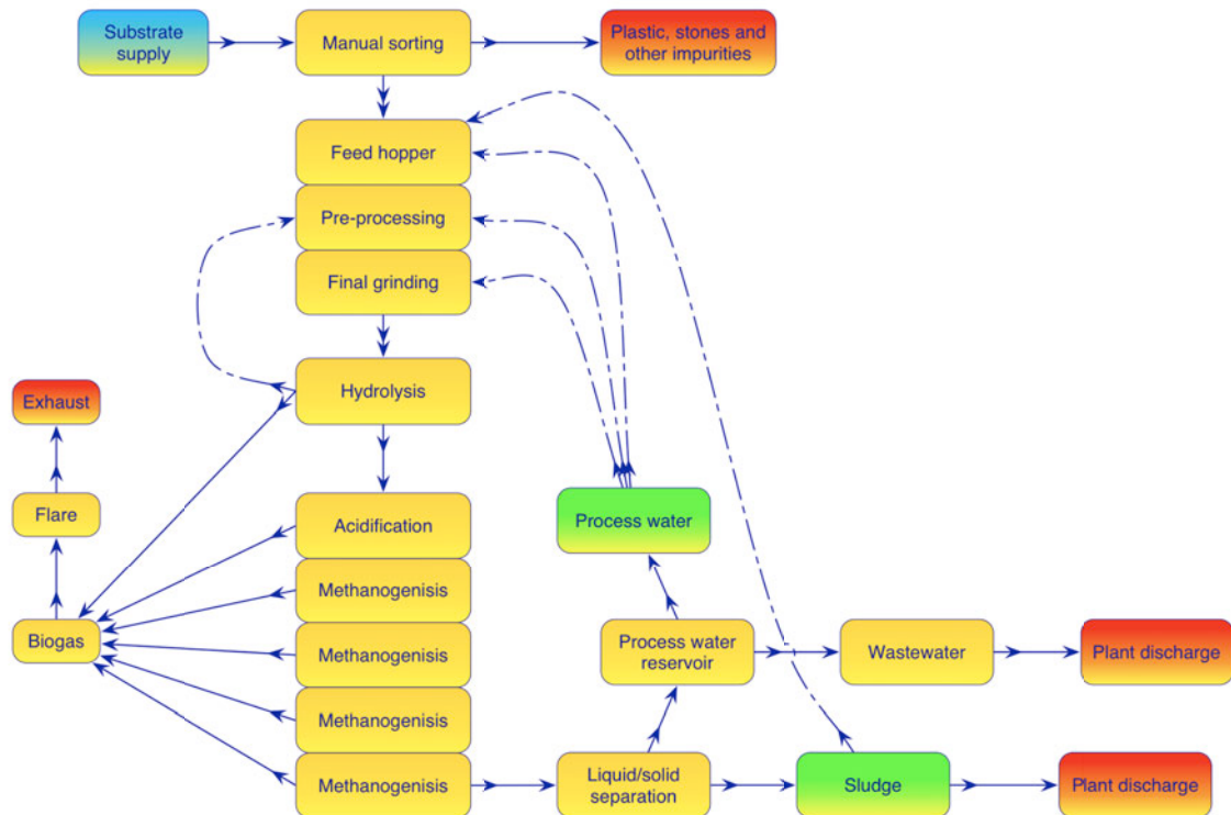
Fig. 61: Continuous cascade biogas digestion process
