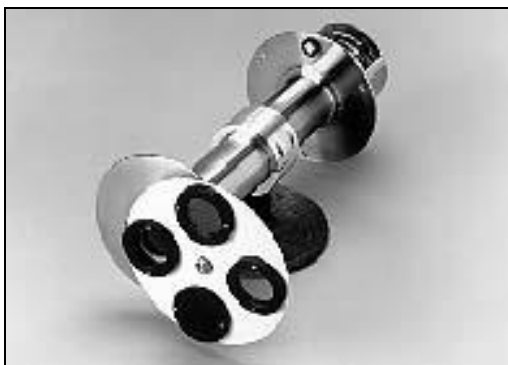
Figure 2.3.5 Eppley Normal Incidence Pyrhelimeter (EPLAP).
