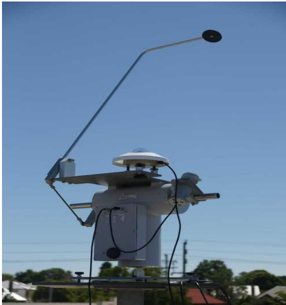
Figure 2.3.4 Middleton Solar-DN5 pyrhelimeter (in active solar tracking system) (Anon)
