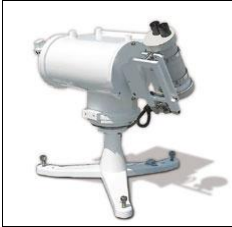
Figure 2.3.6 The EKO-Instrument's Sky scanner MS-321LR (Instruments 2004)
