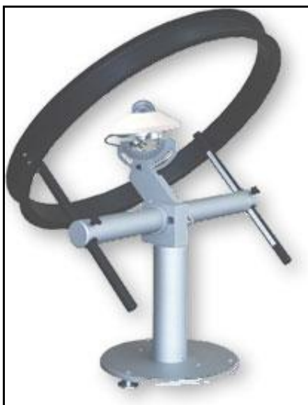
Figure 2.3.2 Kipp & Zonen CM11 Pyranometer with shading device (Clima).
