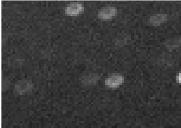
Figure 4.19: An image from a WASP camera with severe focus problems.
