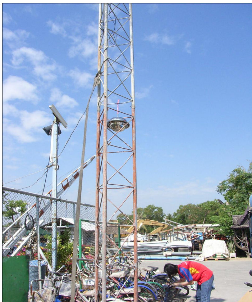
Figure 3.1a PUF disk sampler deployed at outdoor air location*
