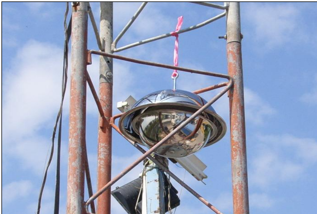
Figure 2.1 PUF disk passive air sampler*
