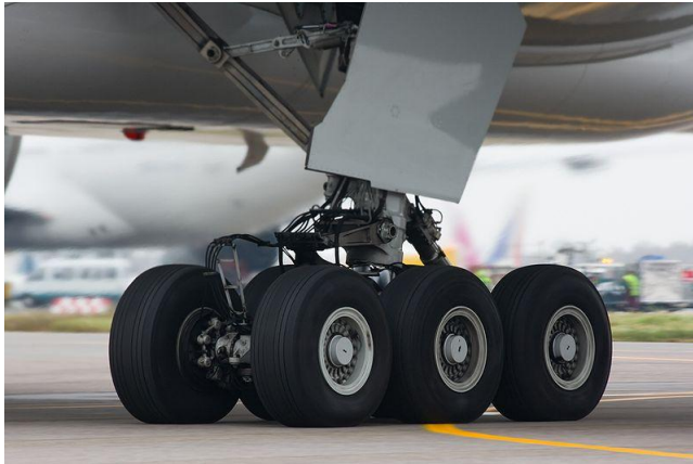
Figure 1.4 – Photo of a retractable landing gear system from a Boeing 777-300 aircraft.
