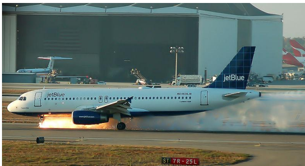
Figure 1.5 – Photo of a JetBlue Airways aircraft making an emergency landing after the front landing gear malfunctioned during take-off.
