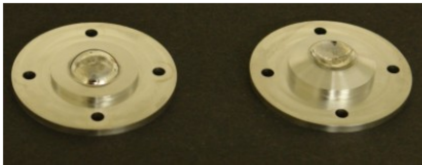
Figure 3.5. The generic metal-on-metal ball (left) and socket (right) sample with 10 mm ball radius
