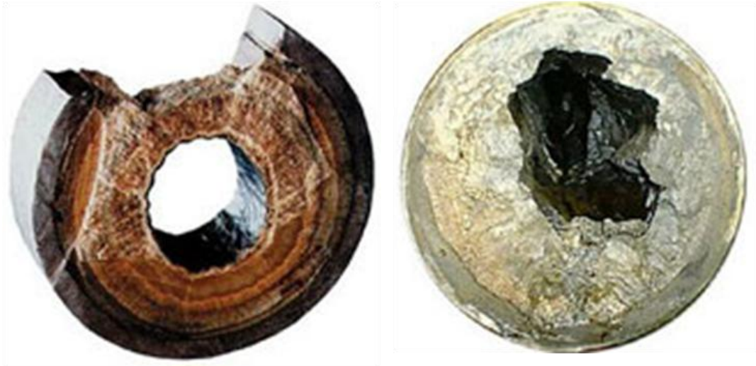
Figure 1.4: Calcium sulphate scaling in oil pipe resulting in significant shrinkage of pipe capacity. 32
