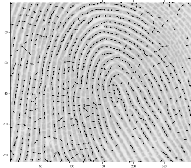
Figure 4.4: Principal eigenvectors of the tensors created by the tensor method (with \sigma_{FO} = 3 ). Lines through each data point indicate the orientation of the principal eigenvector.
