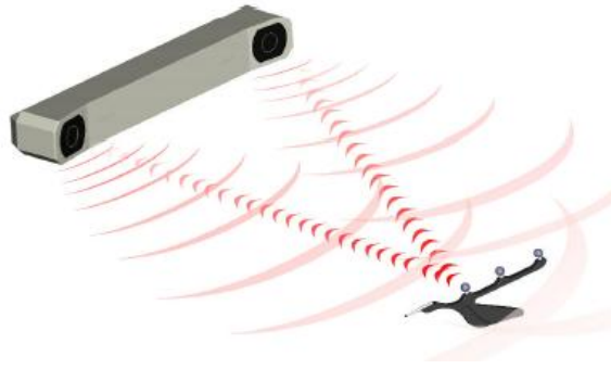
Figure 4.7 Passive markers reflect infrared light back to the position sensor[NDI, 2005].
