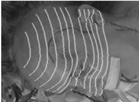
Figure 2.28 Laser scan of a subject's head. Collected laser points are shown as white curves [Ettinger et al., 1998].
