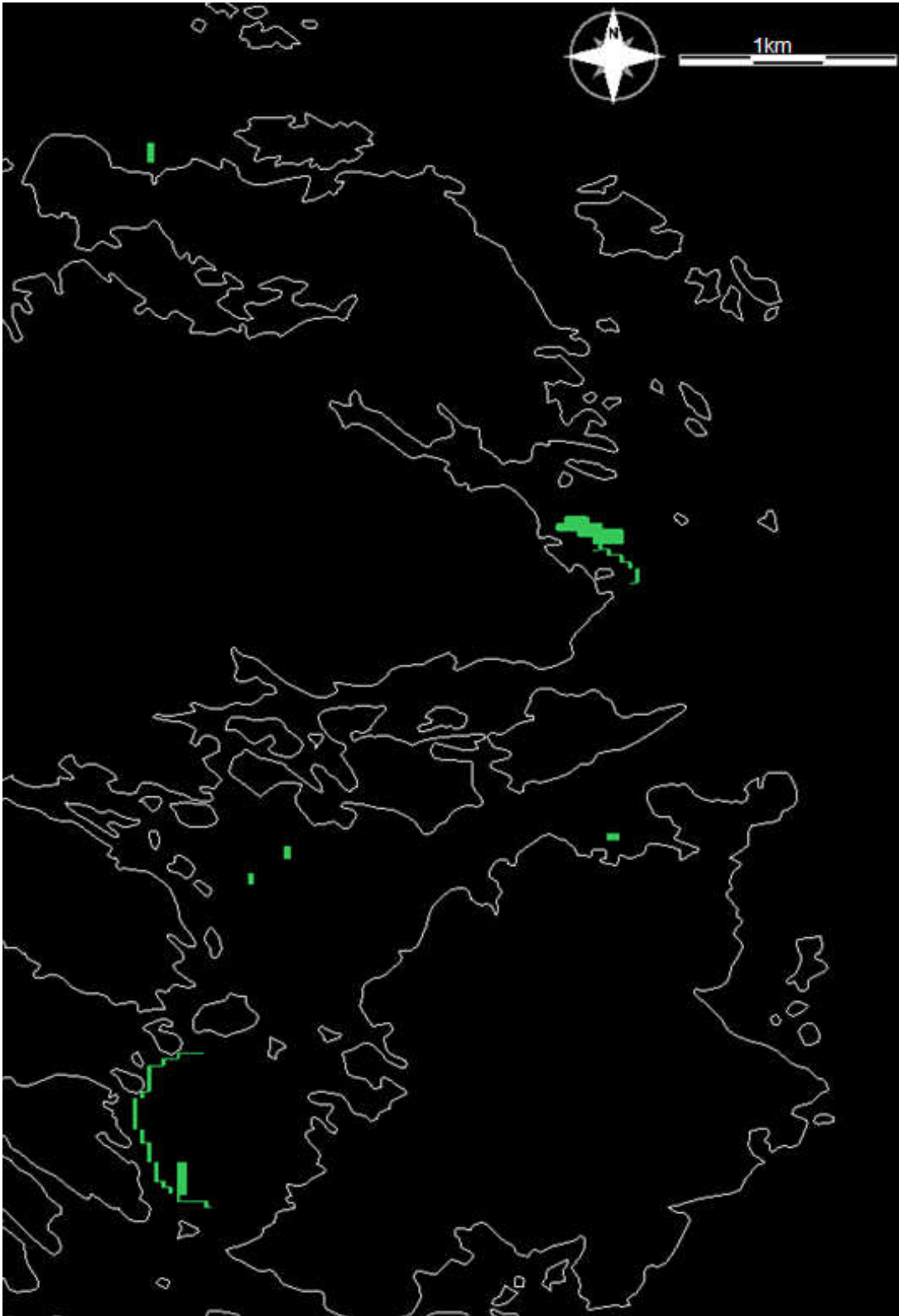
Fig 4.8. GIS-based particulate dispersion model for East Benbecula Fjord system using depth as the forcing image at a resolution of 1m.
