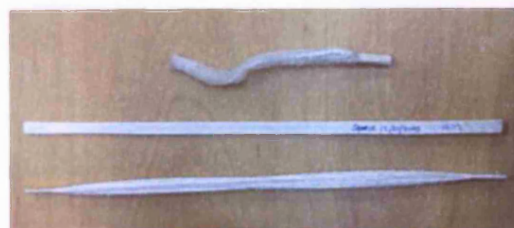
Figure 4.8 - Visual Shrinkage of WPP
