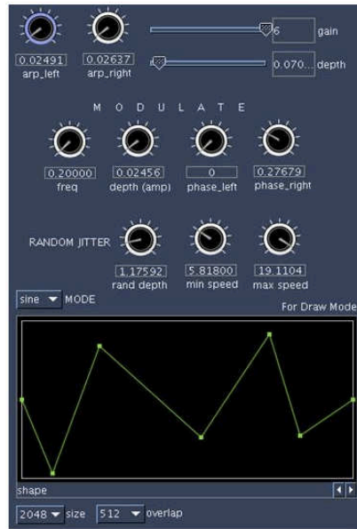
Figure 11. A spectral transformation instrument designed with Csound and Steven Yi's front-end Blue. 194 This instrument allows the introduction of random as well as periodic arpeggiation of the frequency bins with independent control over the left and right channels. 195
