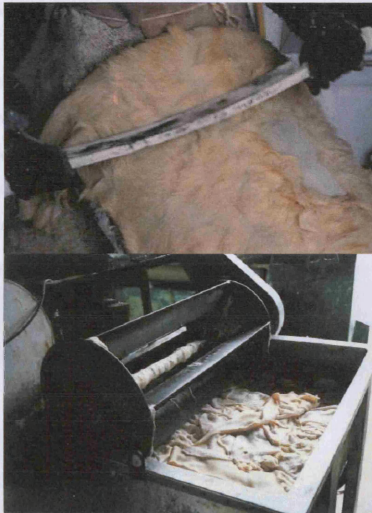
Figure 1.15: Images from the manufacturing process of parchment. Top) Hide placed on wooden beam and hair removed by scraping. Bottom) Mechanical flesher to remove fats, muscle and hair follicles. Images supplied by Linda Ramsay of the National Archives of Scotland. Authorised for publication by Wim Visscher of William Cowley, Parchment works, Newport Pagnell.
