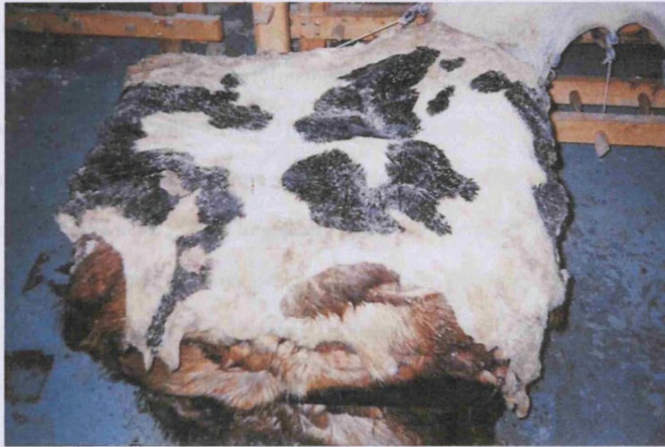
Figure 1.13: Flayed calfskins, salted and stacked together ready for processing into parchment. Images supplied by Linda Ramsay of the National Archives of Scotland. Authorised for publication by Wim Visscher of William Cowley, Parchment works, Newport Pagnell.
