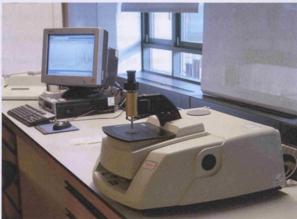
Figure 3.11: Picture of a FT-IR system at the National Archives, London, kindly supplied by Kostas Ntanos and Nancy Bell.
