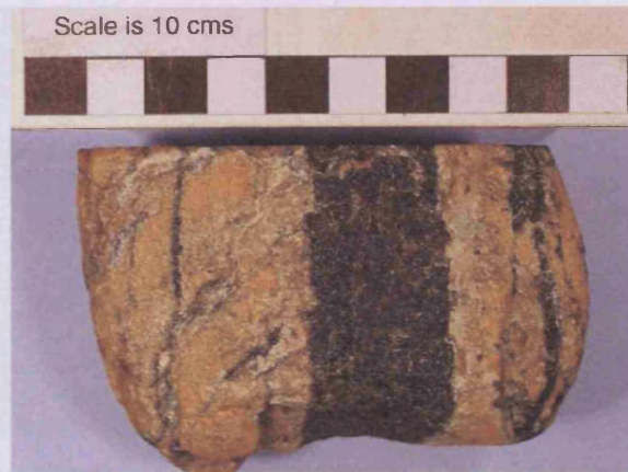
Figure 2.18: Magmatic texture; banded chromitite float from a wadi downstream from a mine in West Zikt, KF-n (sample U.A.E.94).
