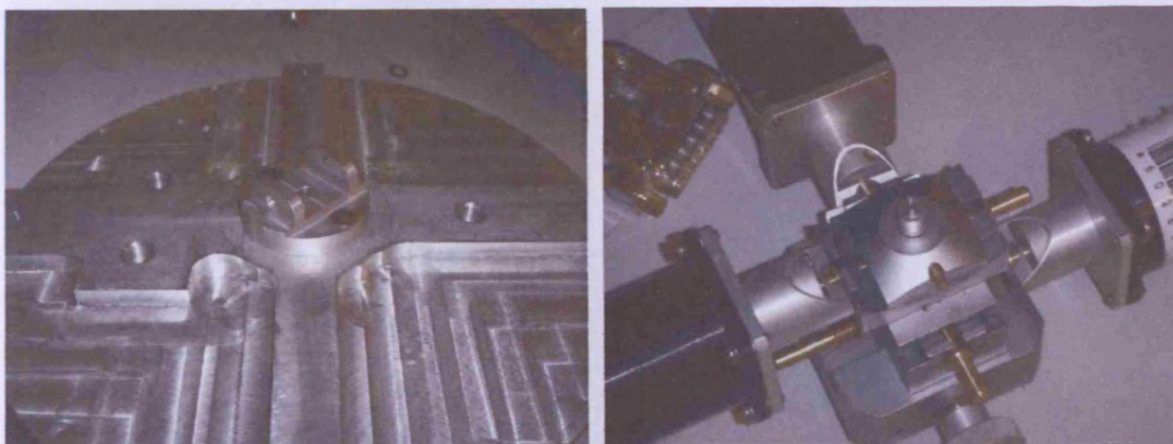
Figure 3.2: The chamber base and the goniometer that attaches it to the diffractometer. Sections of the base have been machined away to minimise the weight of the chamber.
