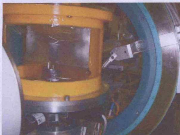
Figure 3.5: The phi rotation clamp allowing the shielding to remain stationary with respect to the beamline as the sample and chamber rotates
