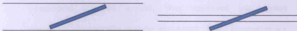
Figure 4.12: Sample illumination, where the beam is larger and smaller than the sample
