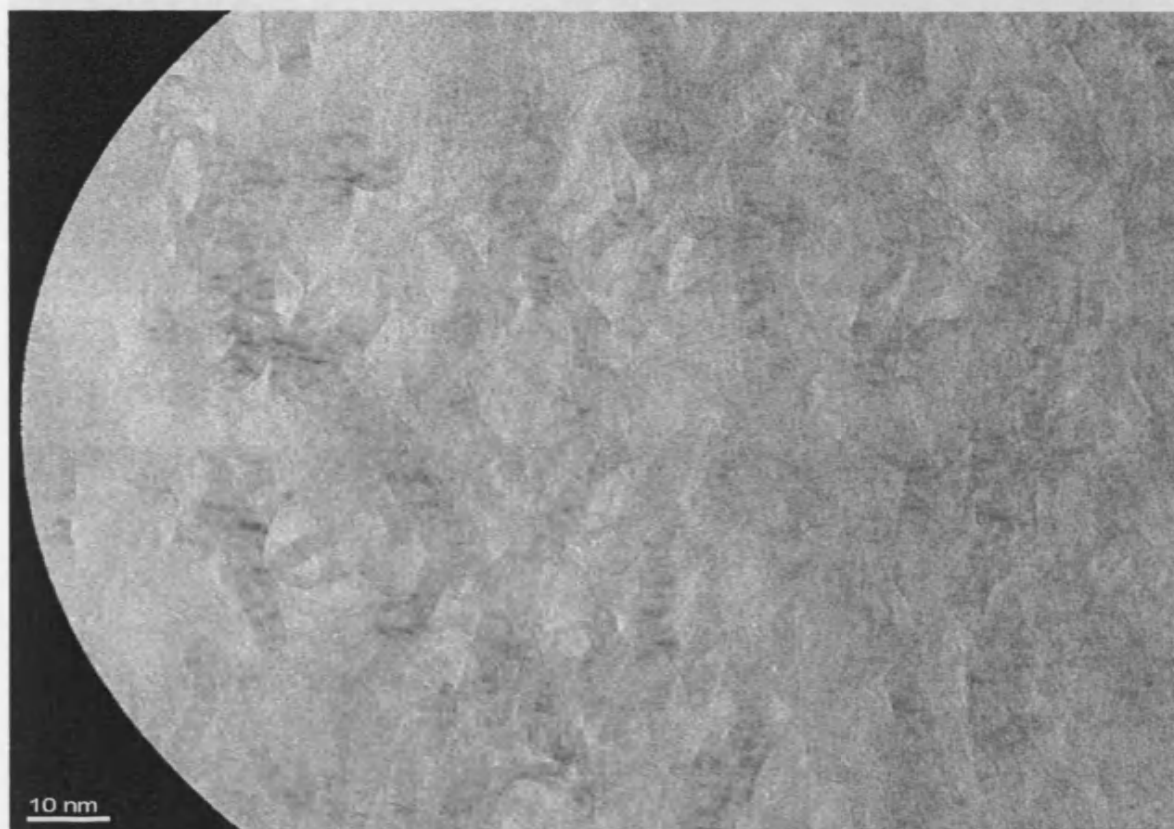
Fig. 5.20: A TEM image of virgin PGA showing the randomly orientated graphitic packets.
