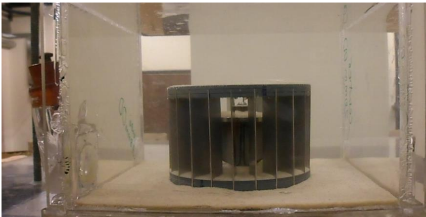
Figure 3.10a: Picture showing settled silica sand when the agitator is stationary
