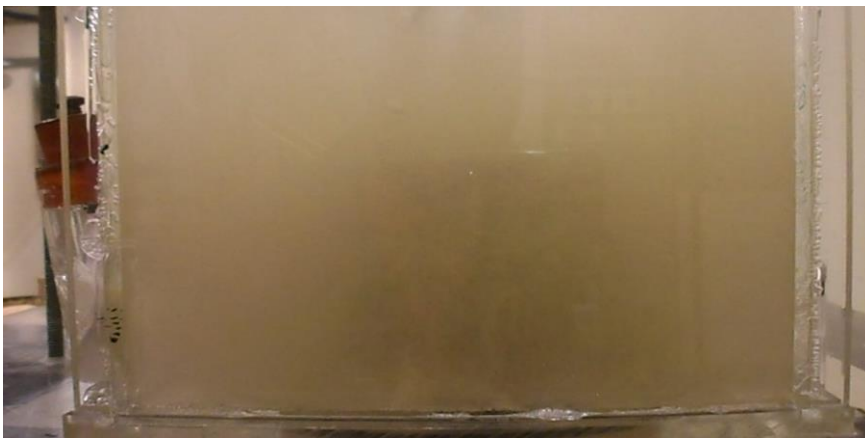
Figure 3.10d: Picture showing all sand particles suspended in the water agitator speed at 2000 rpm.
