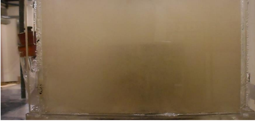
Figure 3.10c: Picture showing almost all sand particles suspended in the water agitator speed at 1500 rpm.
