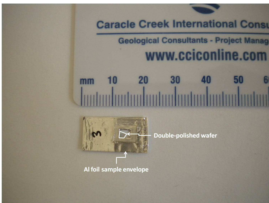
Figure 5.3: Aluminium sample envelope containing a double-polished quartz wafer. The tightly pressed envelope is mounted in a sample ladder that can hold eight samples vertically, which is inserted in to a sample chamber in the nuclear microprobe.
