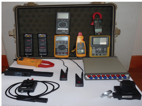
Figure 1 Measurement equipment used for fast recordings on unit
