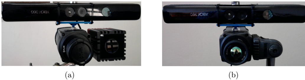
Figure 3.12: The first two iterations of the sensor head: a) with the SR4000 TOF camera and b) without the TOF camera
