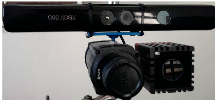
Figure 3.11: The prototype sensor showing the Kinect at the top, the SR4000 on the bottom right and the FLIR A300 in the centre
