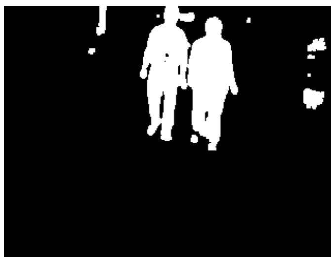
Figure 4: ROIs extracted with the temperature range threshold
