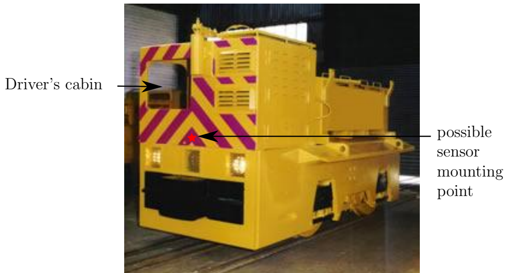
Figure 1.2: An example of an underground locomotive with limited visibility for the driver and a possible mounting point for the thermal imaging-based pedestrian detection system (Adapted from [4])
