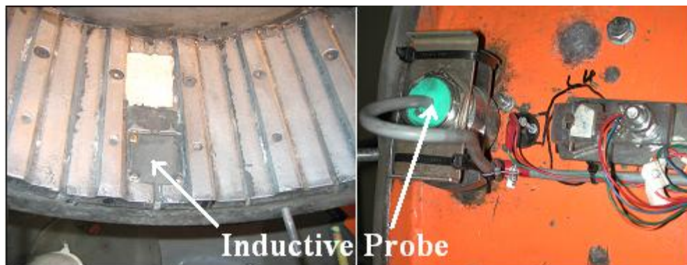
b) Inductive probe installation on the mill
