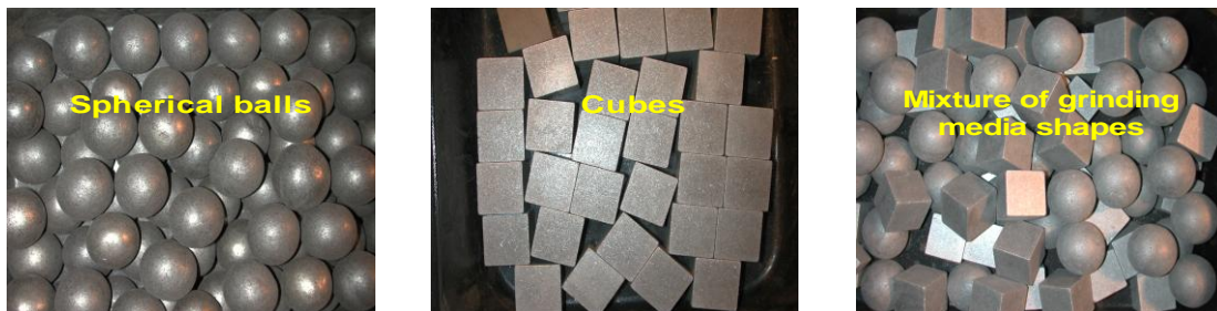
Figure 3.3 Photographs of spherical balls, cubes and a mixture of grinding media shapes used in this study.
