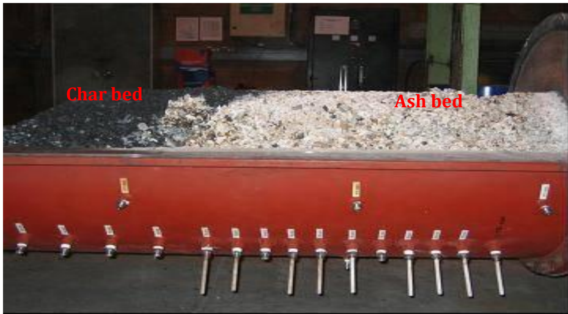
Figure 3.1: A photograph showing the bed profile of the packed-bed reactor combustor unit (left =top of reactor, right = bottom of reactor).
