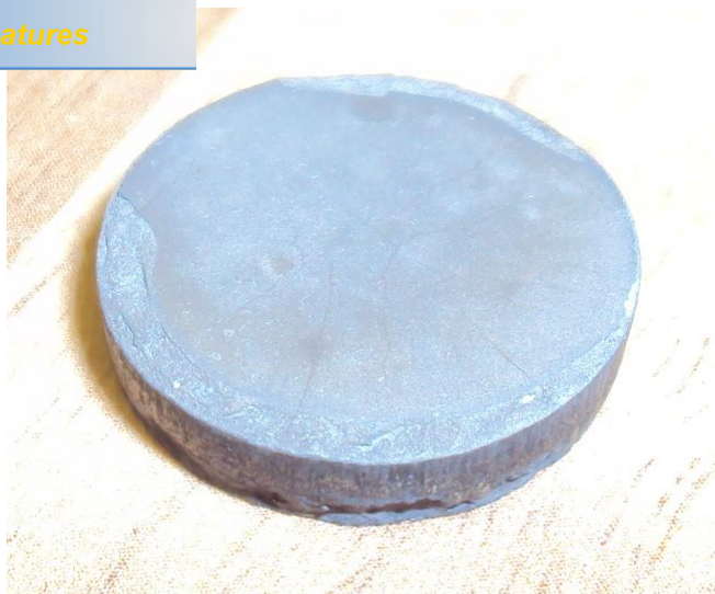
Figure 5. 2: Macrograph of green compact from \text{TiH}_2 powder with broken corner at higher compaction pressure (>393MPa).
