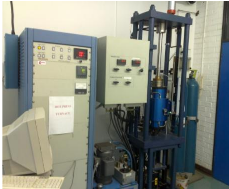
Figure 3. 7: Uniaxial hot pressing machine used for the sintering of composites (HP20-2560-FP20 Thermal Technology)
