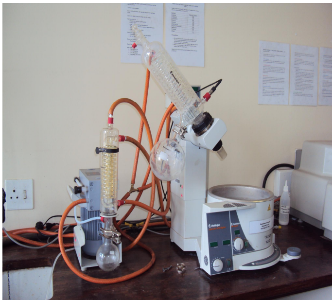
Figure 3. 5: Rotary Evaporator (Heidolph-4010)
