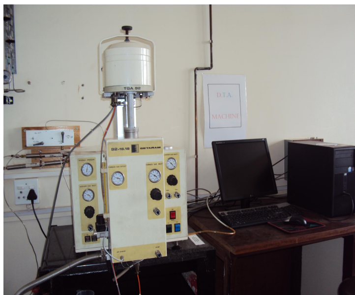
Figure 3. 3: TGA/DTA machine (TG 92 Setaram) (run under argon atmosphere)
