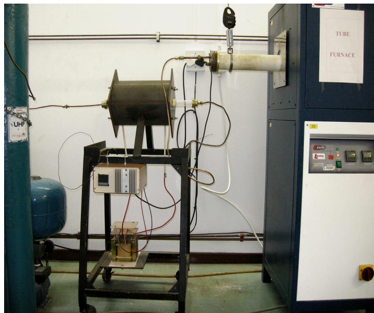
Figure 3. 6: Tube furnace with oxygen getter furnace (Elite TSH17/75/150, Elite Thermal Systems)
