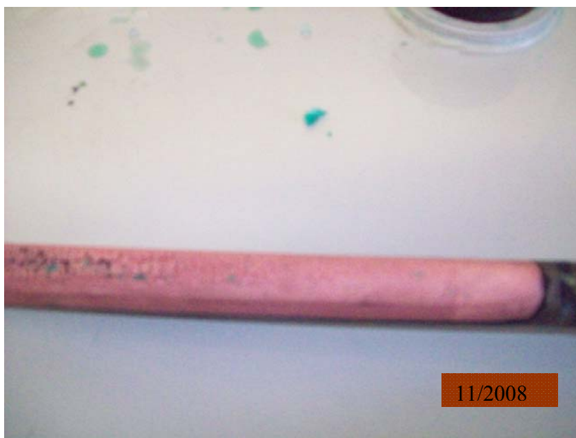
Figure 5.40: Heating Rod Showing Electrodeposited Copper in the Lead Anode Cell.
