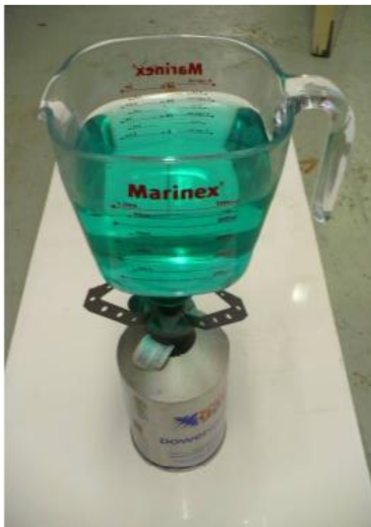
Figure B.4: Electroless nickel solution.
