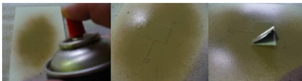
Figure B.29: Masking using spray paint.
