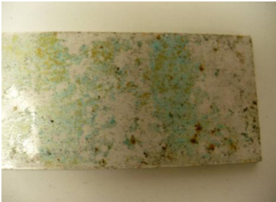
Figure B.7: Very little coverage or adhesion, showing the ineffectiveness of the dilute etching solution.
