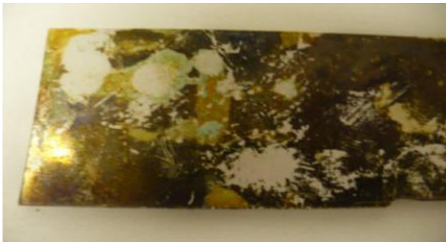
Figure B.8: Test part showing the patchy coverage as well the differences in adhesion on different parts of the polystyrene.
