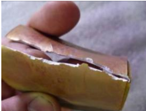
Figure B.27: Bend test after heating.
