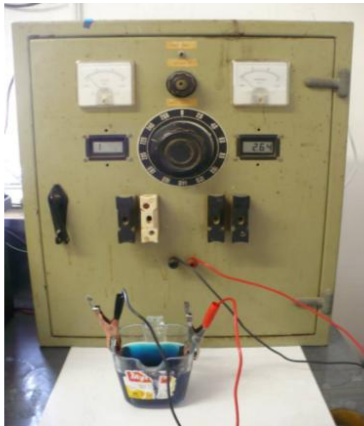
Figure B.16: Rectifier and plating solution.
