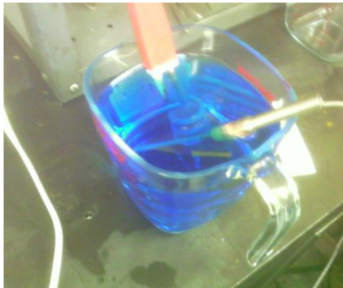
Figure B.2: The glass beaker with the electroless copper solution showing the heating element and the thermocouple.
