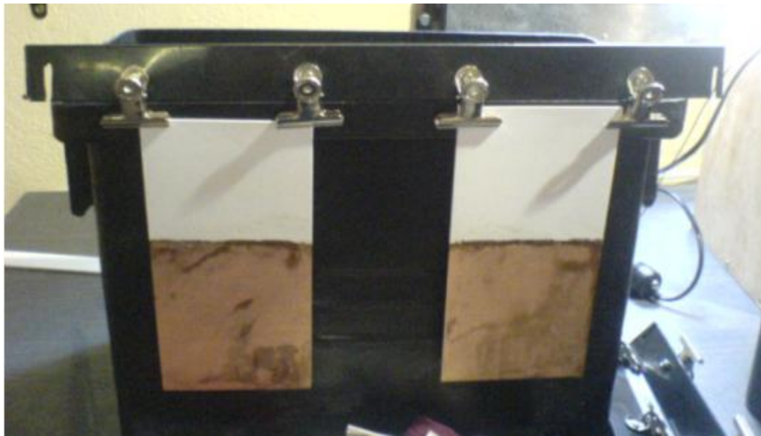
Figure B.17: Two samples plated using the test plating plant.
