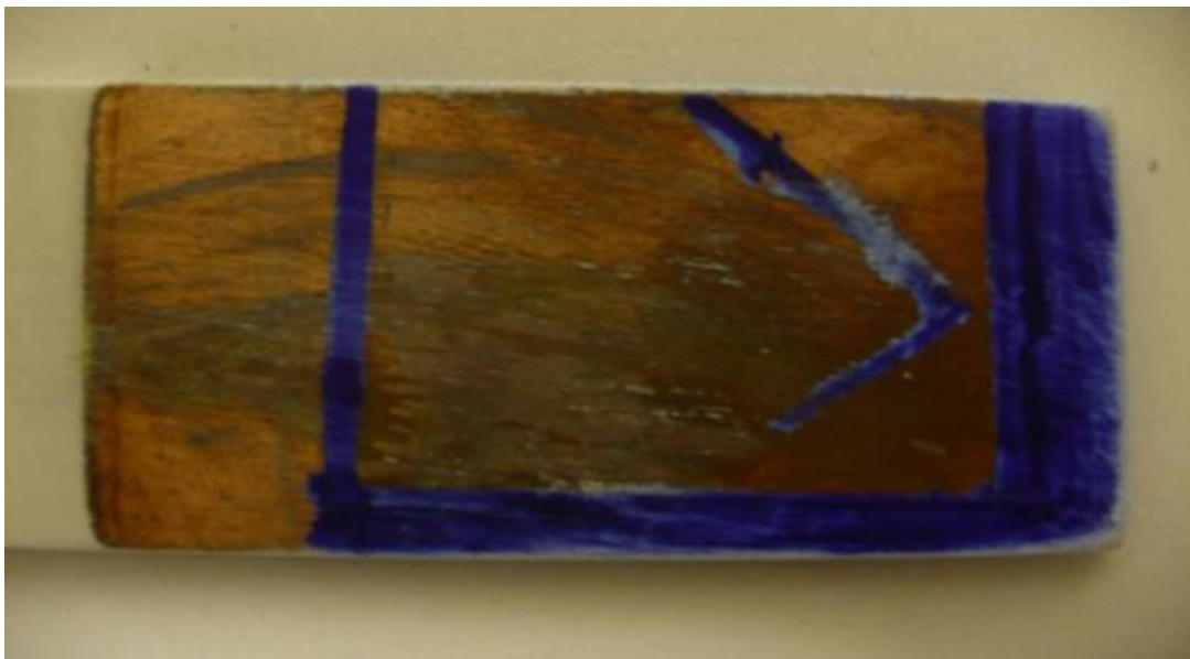
Figure B.28: First basic permanent marker masking test.
