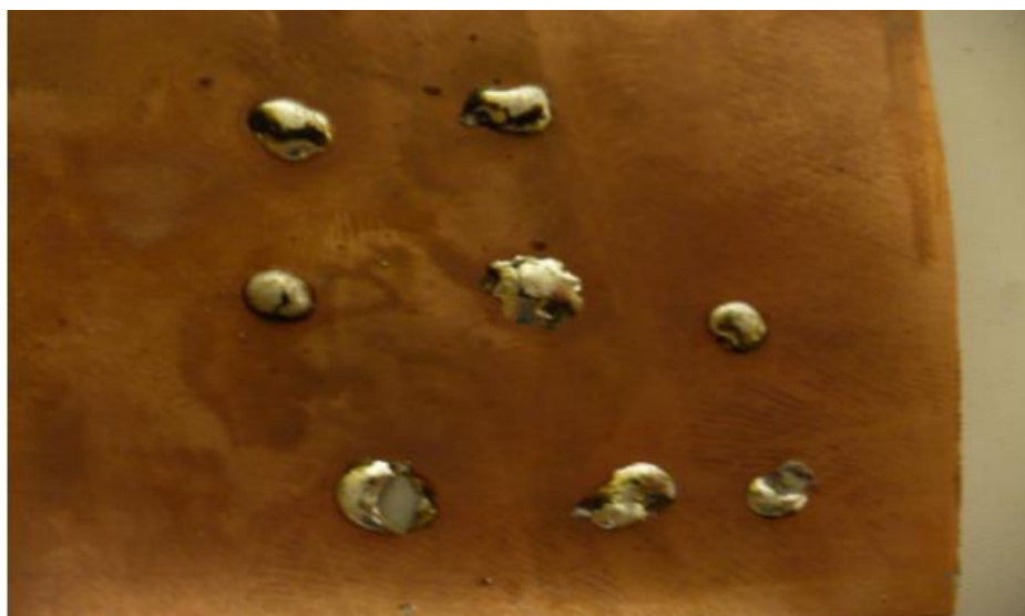
Figure B.22: Electroless plated sample being soldered. If the solder is applied quickly then the copper does not burn away.
