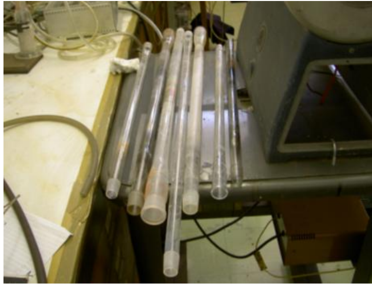
Figure A.3: Examples of the quartz reactors.
