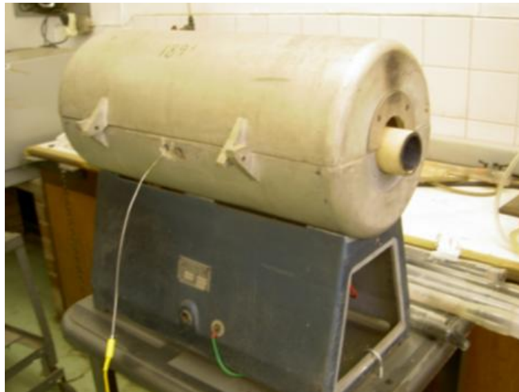
Figure A.4: Furnace used to produce carbon nanotubes.
