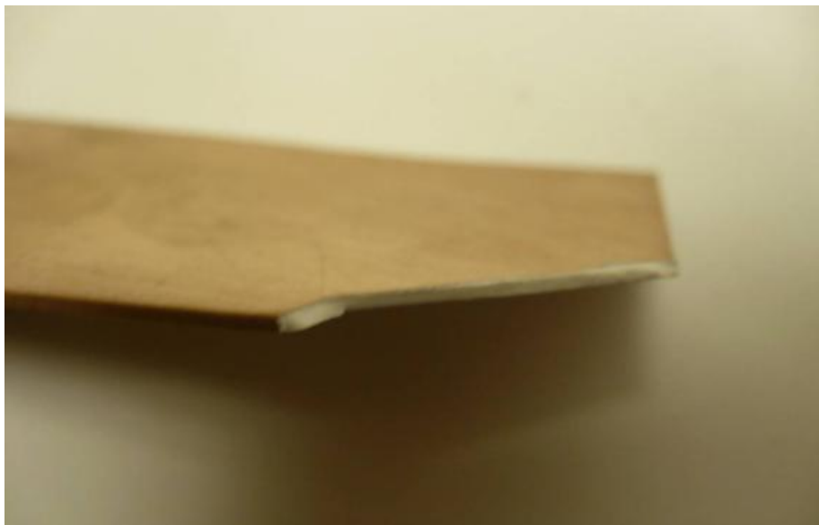
Figure B.20: Later sample with torn corner shows the straight tear of the copper, with no peeling.
