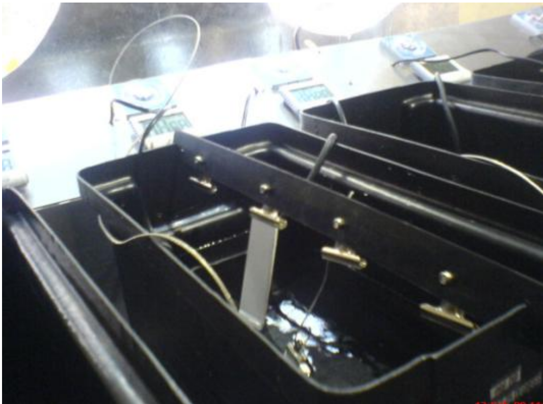
Figure B.14: The pre-dip tank with a test sample held by the jig.
