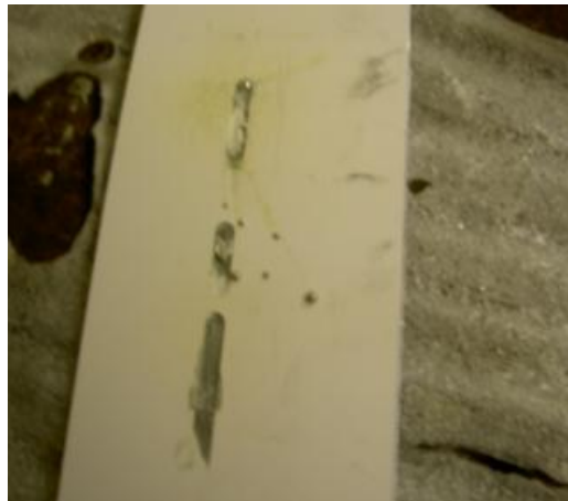
Figure A.14: The solder paste coagulates in the surface indentation.
