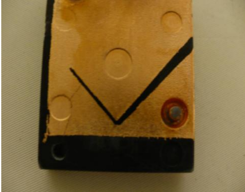
Figure C.1: PIFA antenna prototype.
