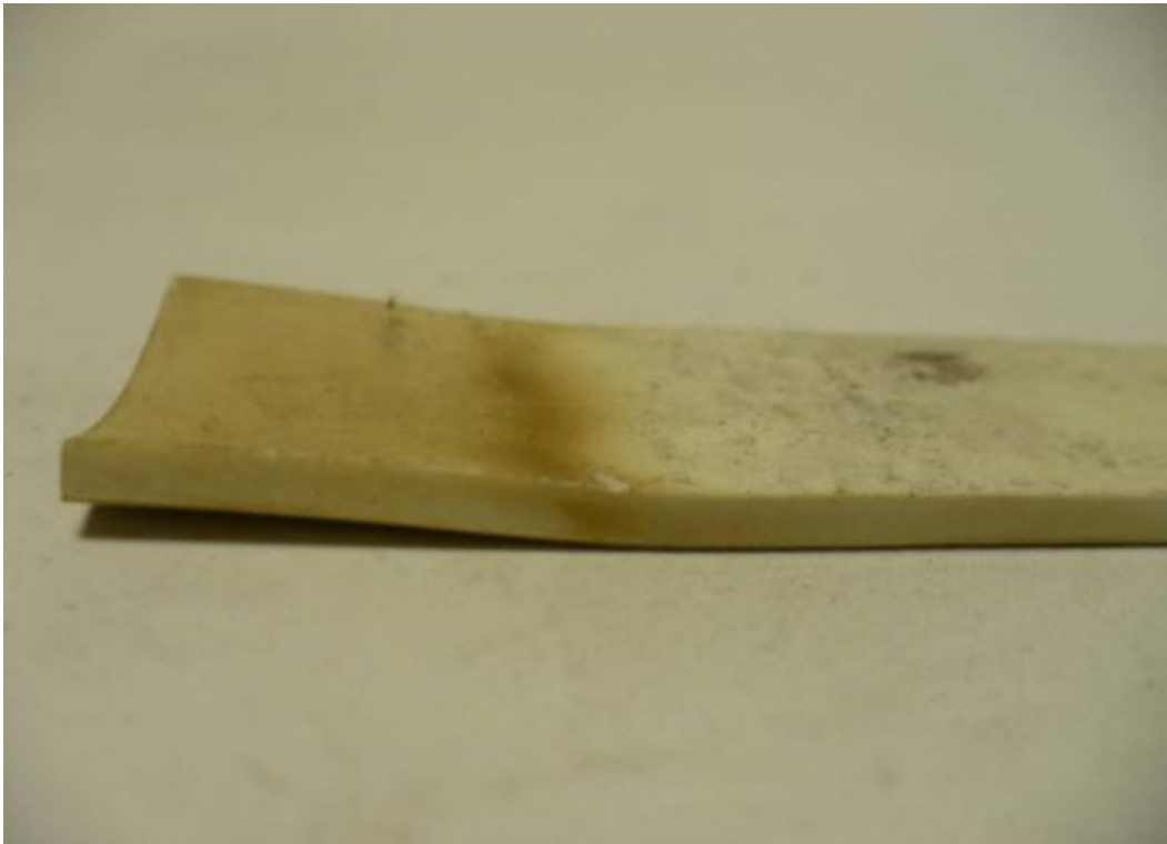
Figure B.9: The sulphuric acid and hydrogen peroxide solution when recently mixed causes the polystyrene to warp at high temperatures.
