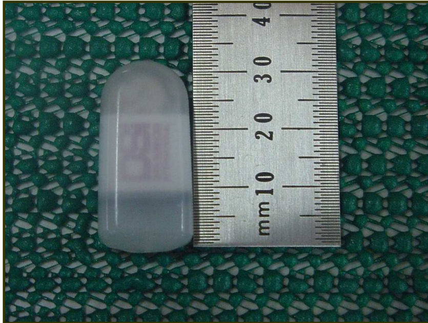
Figure 1. A temperature-sensitive radio telemeter which was inserted into the rat abdomen.
