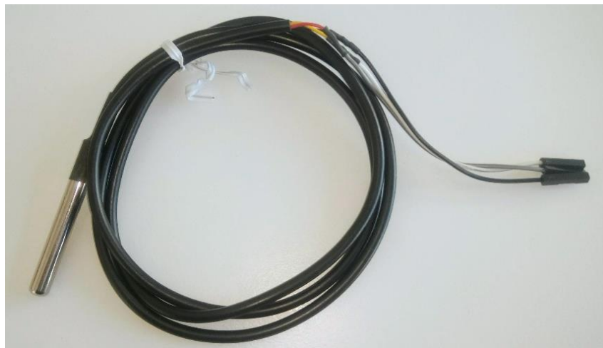
Figure 4.2 – Temperature sensor DS18B20.
