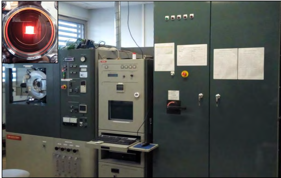
Figure 2.1. Dr. Sinter 2080 Spark Plasma Sintering unit
