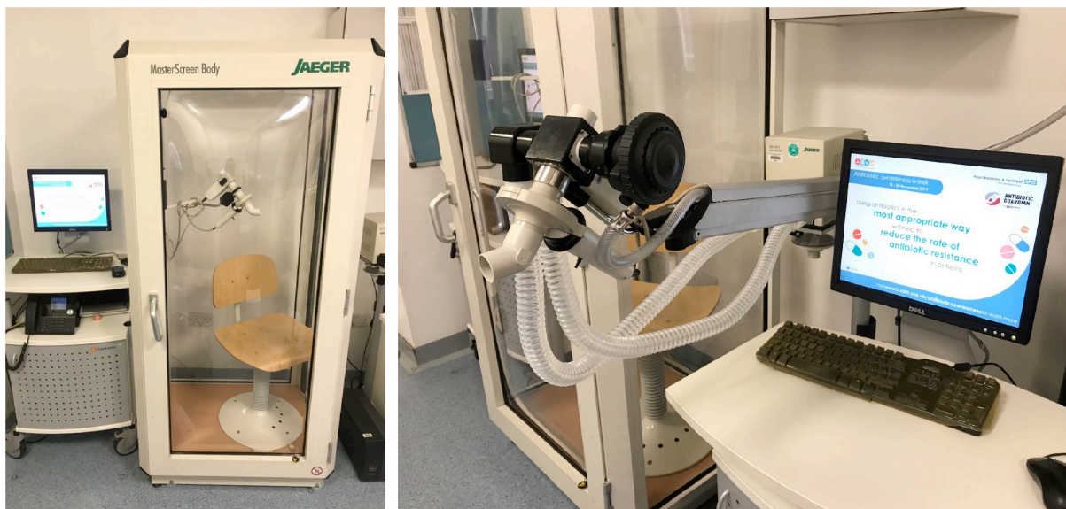
Figure 2.2. Whole body plethysmograph (left) and Single breath gas transfer unit (right).
