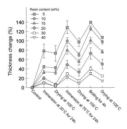
Fig.8. Thickness change in a cyclic accelerated aging treatment. Error bars indicate standard deviations
