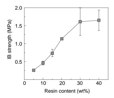
Fig.7. Effects of resin content of citric acid / sucrose on IB strength. Error bars indicate standard deviations
