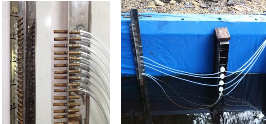
Figure 2.26 Rising stage suspended sampler installed at the outlet of catchments A, B, and C.
