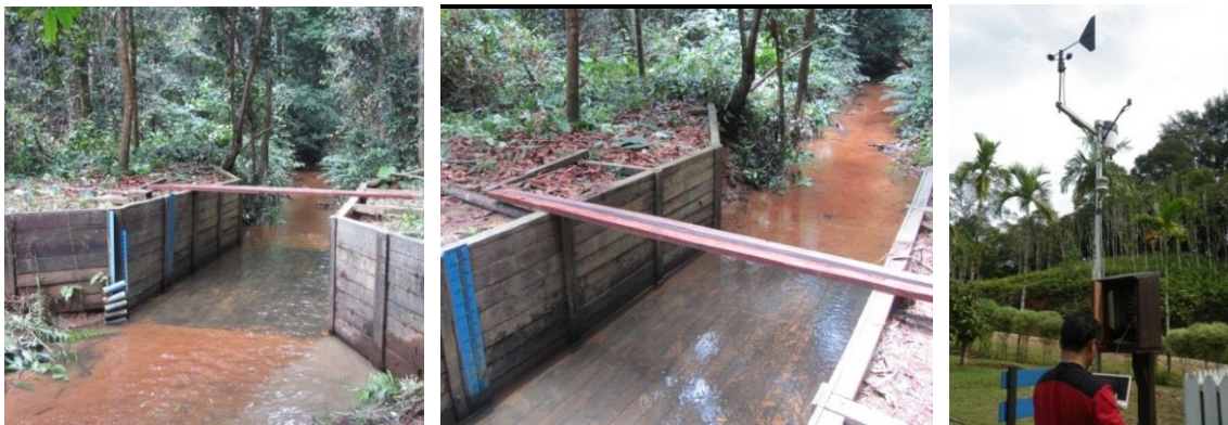
Figure 2.19 Flume weir in the C2 outlet and the weather station.
