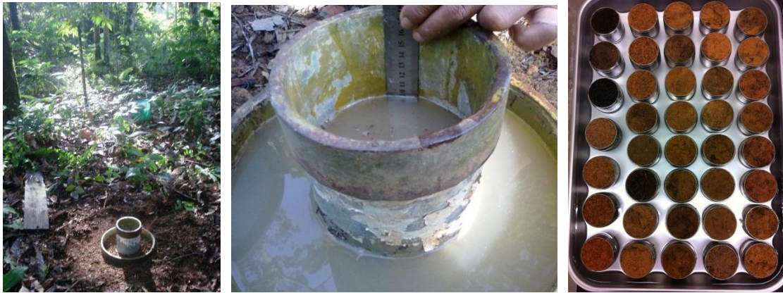
Figure 2.13 Infiltration test and preparing soil sample test for saturated hydraulic conductivity.
