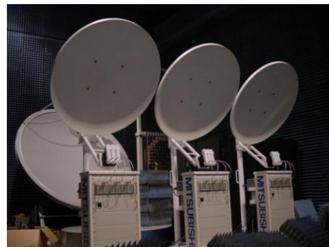
Fig.14 Parabolic phased array using DDS/PLL oscillators.
