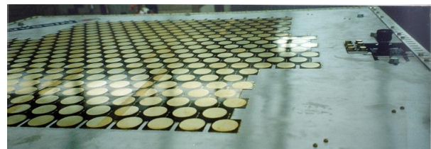
Fig.3 First phased array used for a MPT application for the MILAX in 1992
