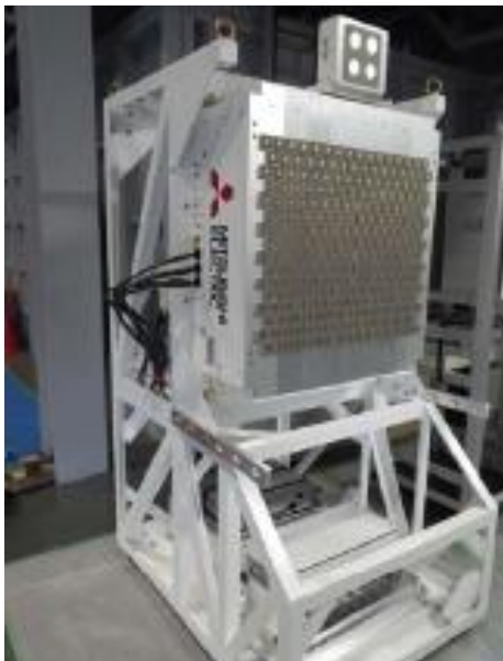
Fig.22 New phased array for MPT with GaN FET and F-class amplifier circuits installed in Kyoto University and developed by Mitsubishi Electric Corporation in FY2010
