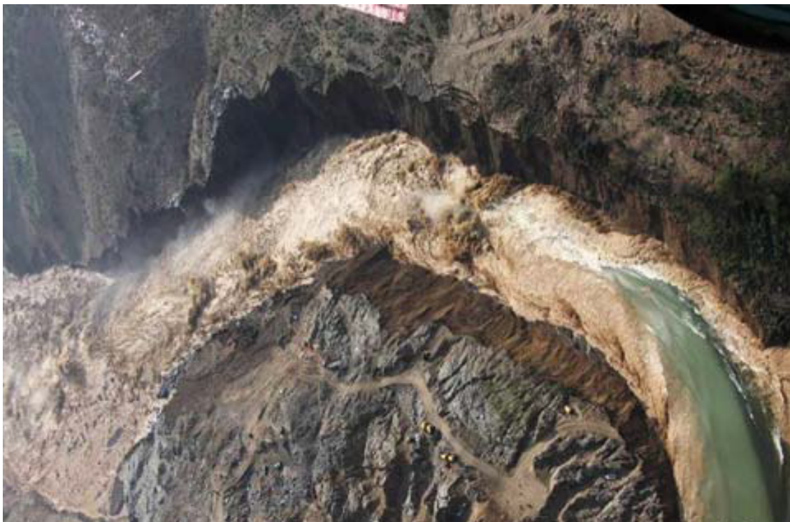
Figure 1.2 Impounded water flowing through the artificial spillway, taken at 11:00 (Beijing time) 10 June 2008 when the discharge reached its maximum (Source: Liu.,2008)
