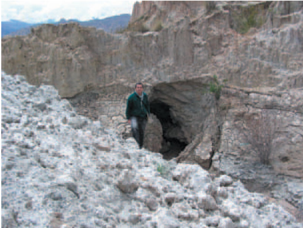
Figure 1.5 Natural water-escape tunnel through a landslide dam in Allpacoma valley, La Paz, Bolivia, formed due to piping failure.
