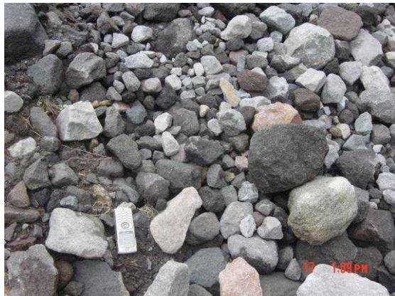
Photo 1.2 Riverbed condition and bed material in Senowo River after sand mining.
