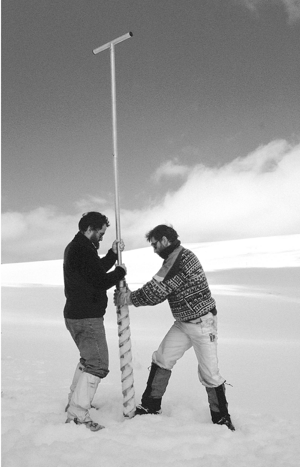
Photo 1: Manual vertical ice-core drilling machine. The ice-cores are extracted in fragments of less than 1 m in length.
