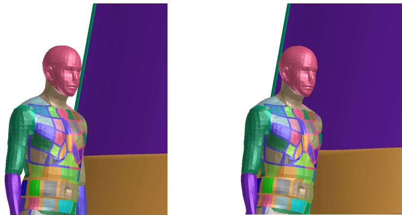
Figure 13. Results of simulation (in time 0 and 25 ms) where the head impacts the windshield.
