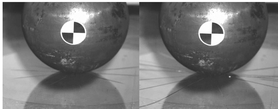
Figure 4. The radial crack propagation after the first contact of impactor.
